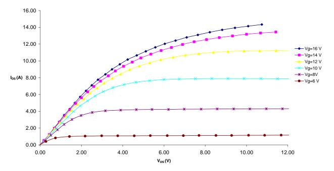
Figure 4 – Typical IV Characteristics.
